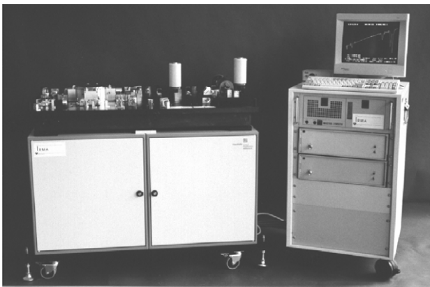
Figure 26. Photograph of the IRMA system: left—optical table, right—data acquisition rack with diode laser controllers and industrial computers [24].
