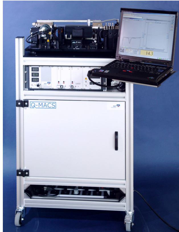
Figure 32. Photograph of the Q-MACS-Trace system with optical arrangement and laptop for analysis. (1 channel system with 56 m long path cell, sensitivity: ppb [131].)
