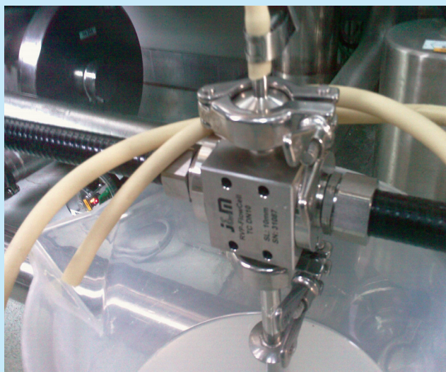
Fig.1: Online installation for cleaning validation in a pharmaceutical plant.
