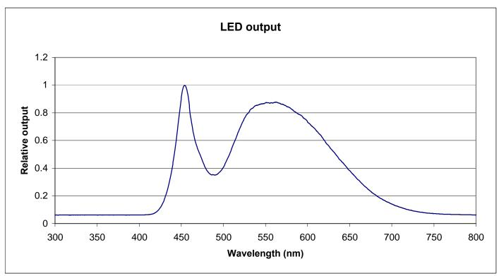
Total measured Output: 2.77 mW
