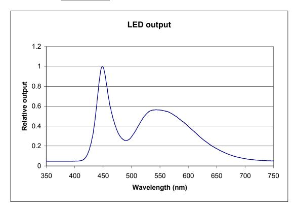
Total measured Output: 4.48 mW (coupled into 600um .22NA fiber)
