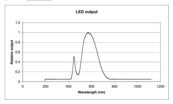
Total measured Output: 1.29 mW
