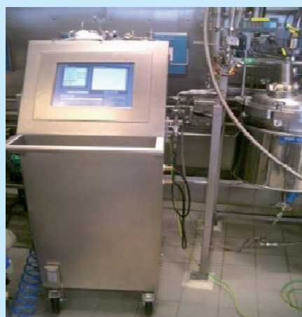
Fig. 3: Typical mobil CIP process analyzer J&M detector inside
