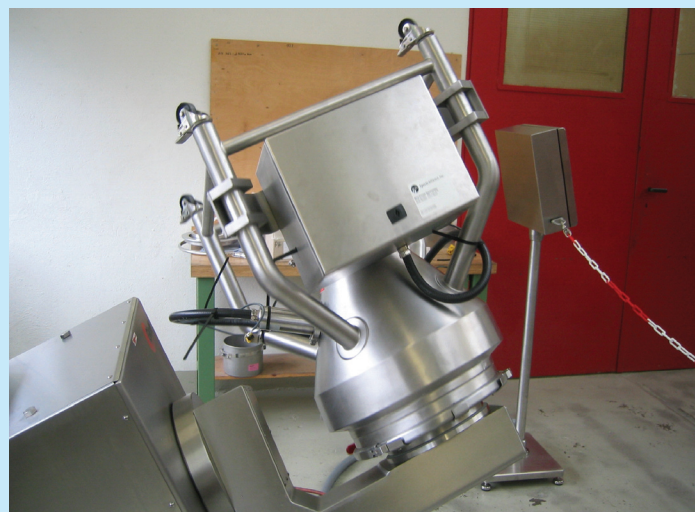
Fig. 2 and 3: J&M process spectrometer (NIR) attached to different blenders.
