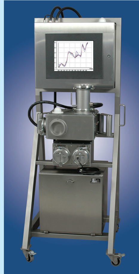
Fig. 4: Detachable NIR Spectrometer mounted on a mobile rack
